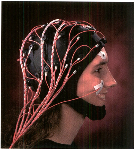
Quik-Caps permit rapid, accurate application of 128 or 256 channel electrode arrays.
