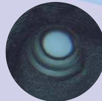
Close-up of electrode cup shows reservoir with gel.
