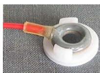
The electrodes are snapped into the adaptors
